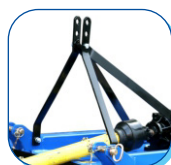
MOUNTED WITH 3 POINTS LINKAGE FOR EASE OF OPERATION
