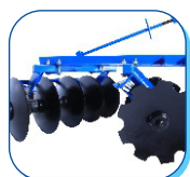
COMBINATION OF PLAIN & NOTCHED BORON STEEL DISC
