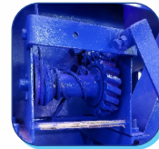
DISCHARGE CHUTE ADJUSTING ROPE HELPS IN ADJUSTING THE OUTLET POSITION AS REQUIRED
