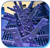
TOUGH THRESHING SPIKES FOR EFFICIENT THRESHING OF GROUNDNUT
